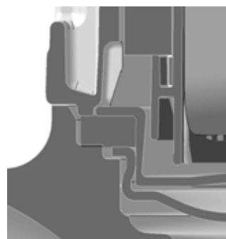
Fig. 37 Sectional drawing showing sealing principle of gasket
