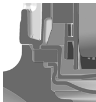
Fig. 37 Sectional drawing showing sealing principle of gasket
